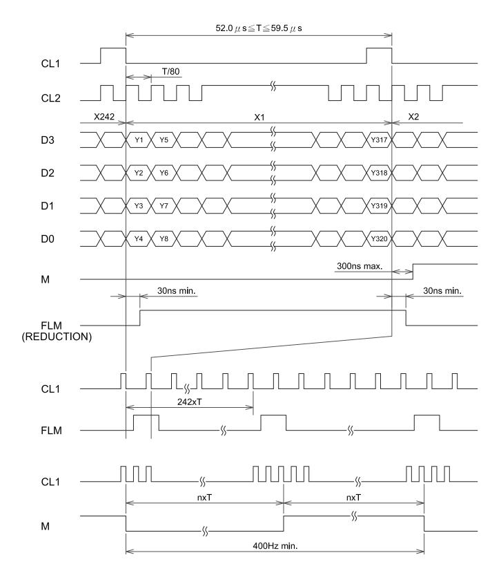
Note 1: M signal should be kept 400Hz min. and 50% duty.
