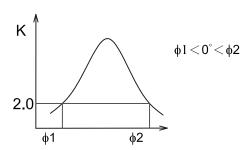
Contrast ratio K vs viewing angle  $\phi$
