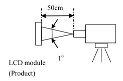
Luminance Meter (TOPCON BM-5A) Spectroradiometer (TOPCON SR-3)
