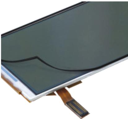
When optical bonding is not practical for your LCD, AGDisplays offers tape, or perimeter, bonding. Perimeter bonding helps your company save on costs while still sufficiently ruggedizing your panels. Our tape bond services provide a secure bond that increases LCD flexibility, long-term durability and improved appearance. The adhesive offers a wide temperature specification, allowing a durable integration method in various environments.
