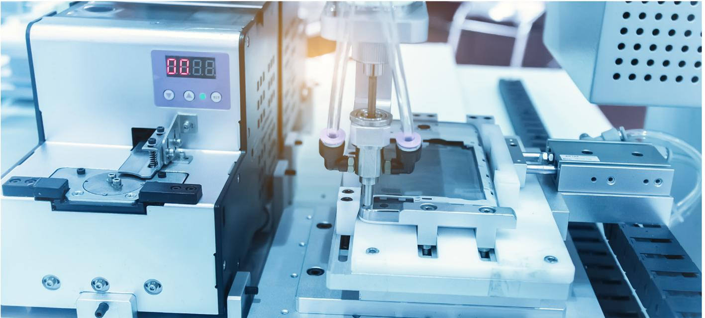
**AGDisplays offers three different methods of bonding for your LCD to add strength and clarity, as well as using it as an integration method when incorporating one of our other value add services. In performing a bonding procedure on your LCD, your display will be more rugged and less prone to environmental vulnerabilities such as dust collection and moisture condensation.**
