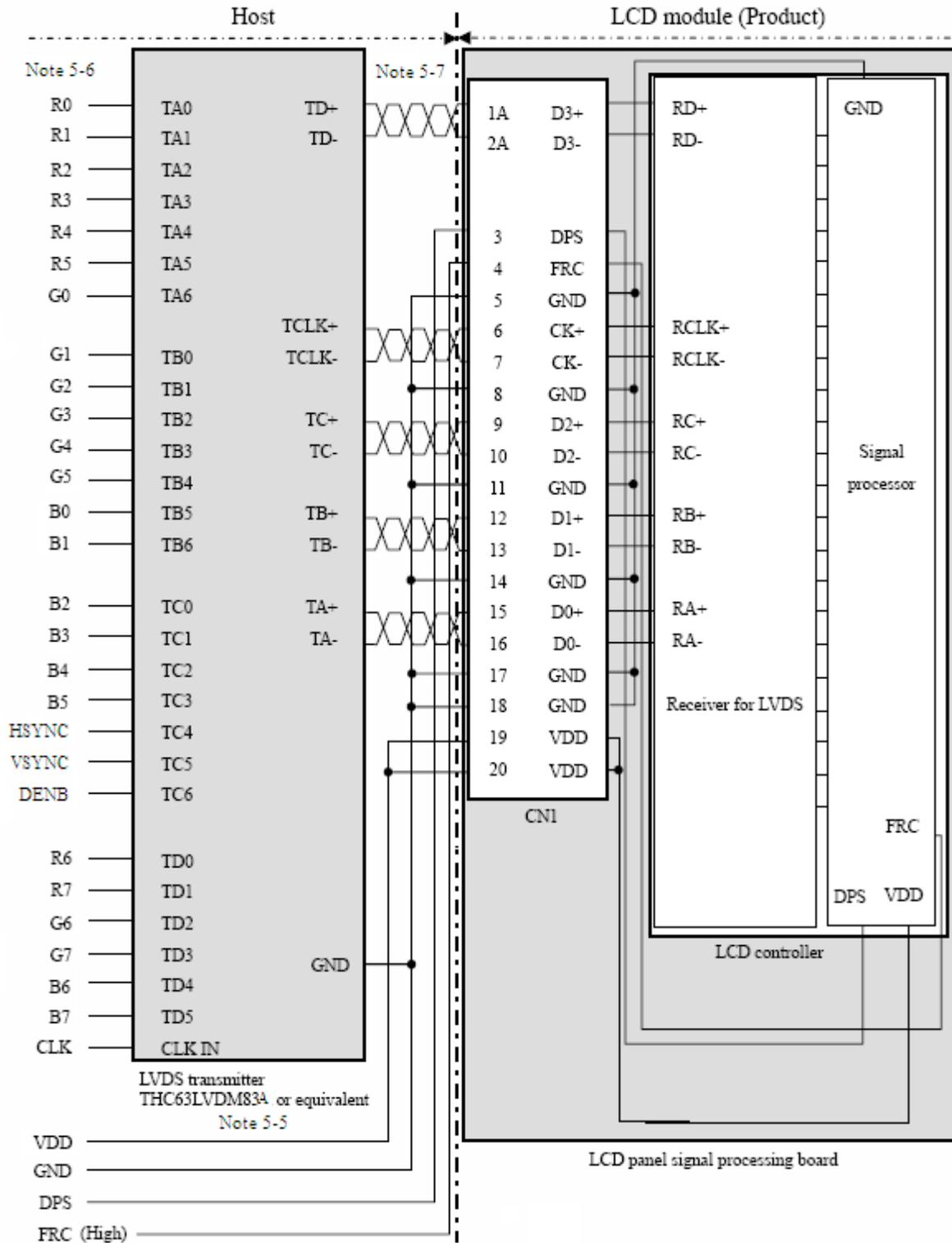
Note 5-5 : Recommended transmitter THC63LVDM83A (THine Electronics Inc.) or equivalent
