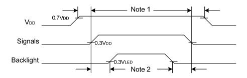
Fig. 9.6 Power Sequence Timing
