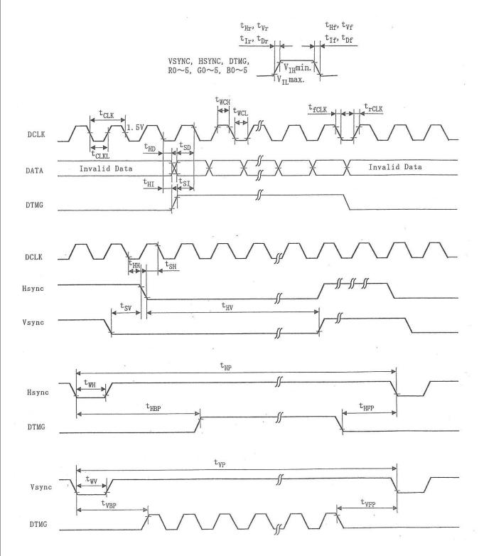
\*The DTMG signal for this module is defined as above-mentioned timings for Vsync and Hsync.
