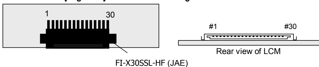
[ Figure 4 ] User Connector diagram
