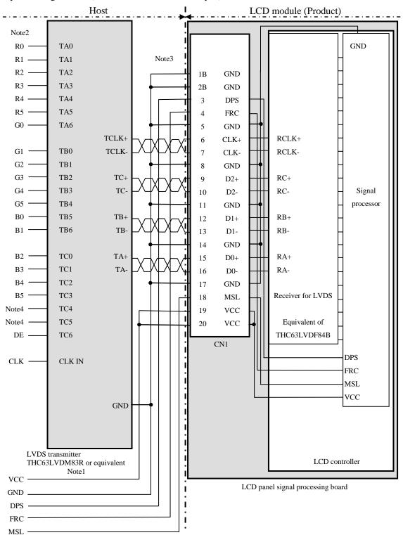
(3) Input data signal: 6bit (MSL: Low, FRC: Low or Open)
