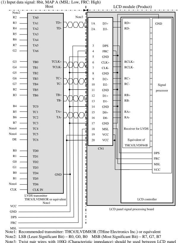
Note3: Twist pair wires with  $100\Omega$  (Characteristic impedance) should be used between LCD panel signal processing board and LVDS transmitter.
