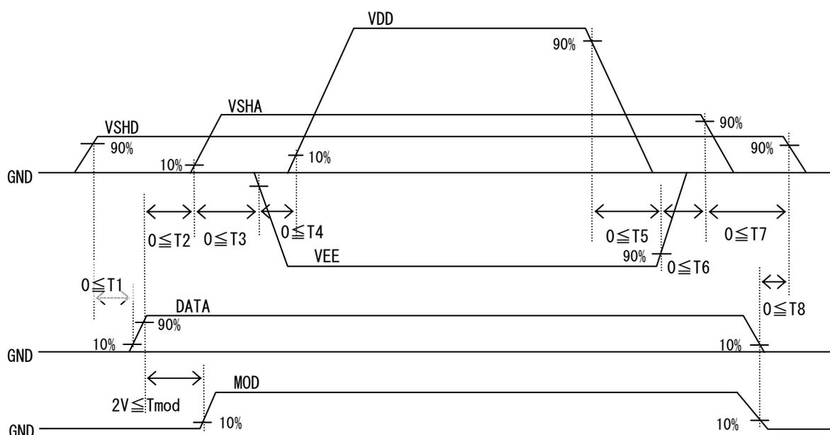
【Note 7-1】 DCLK,SPL,SPR,LBR,LP,PS,REV,R0~R5,G0~G5 and B0~B5 terminals are applied.
