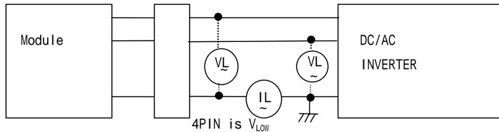
[Note6-2] The voltage at the output of inverter circuitry.
