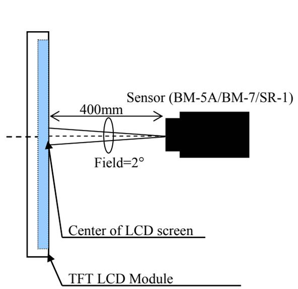
Fig.9-2 Measuring setup for Luminance, Chromaticity and Response time (BM-7 is used for Luminance, SR-1 is for response)
