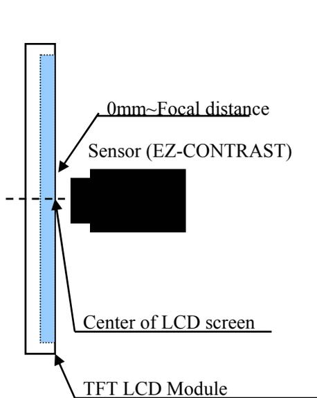
Fig.9-1 Measuring setup for Viewing angle and Contrast ratio (BM-7 is used for contrast.)
