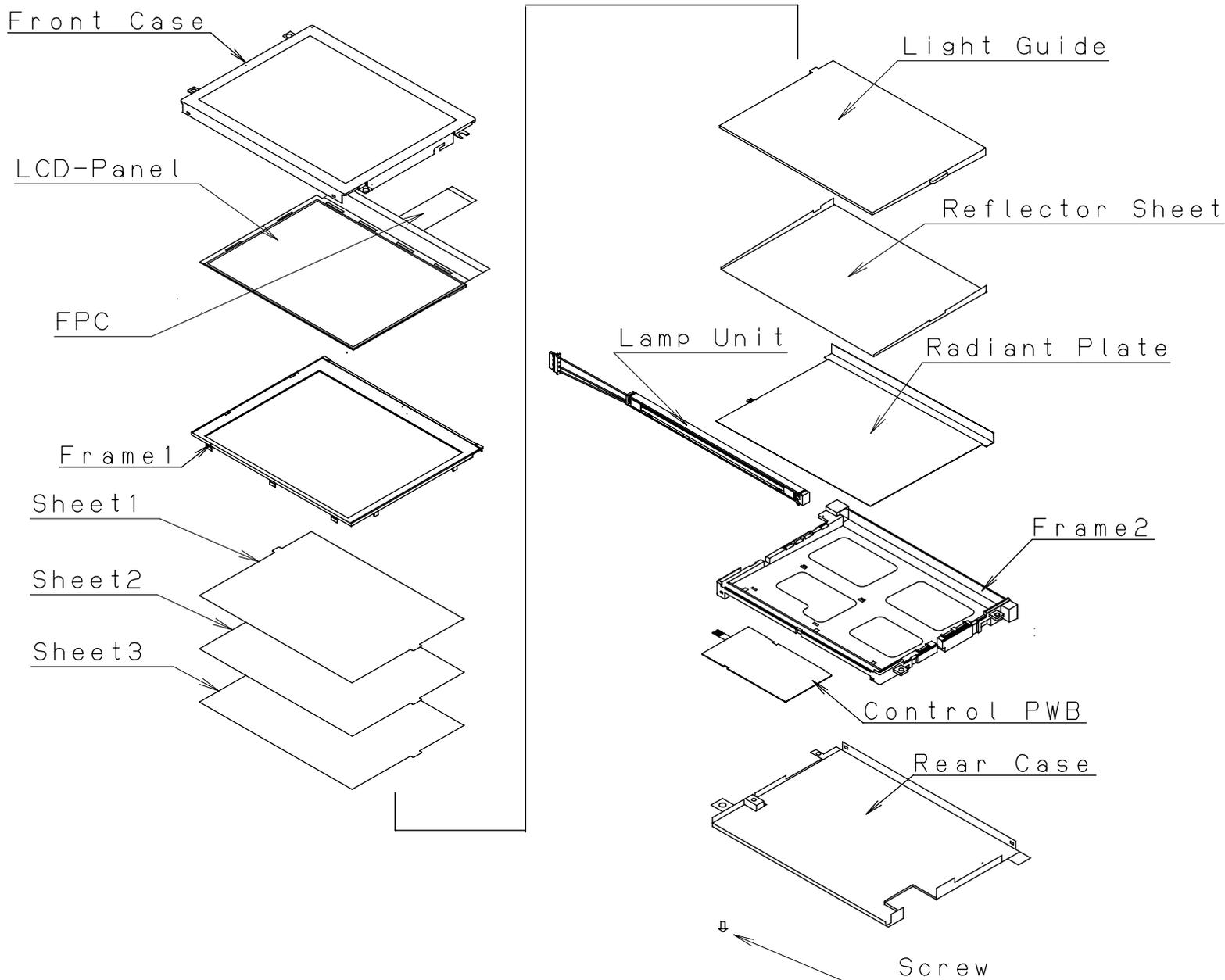
Fig 4 MODULE STRUCTURE
